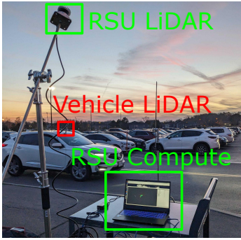
Figure 13: VRF deployment setup.
