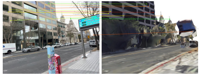
Figure 6: Cross-modality matching between a camera image and an image from an aerial mesh results in relatively few matches.
