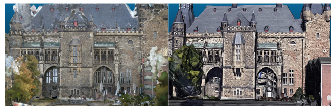
Figure 7: An image rendered from a terrestrial mesh (left) and from an aerial mesh (right). Notice the distorted arch on the right side of the aerial mesh image.
