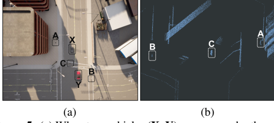
FIGURE 5: (a) When two vehicles ( X , Y ) are near each other, after ICP, RECAP can find the relative position of pedestrians A , B and C and obtain a denser point cloud of C . (b) Generated point cloud.
