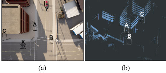
FIGURE 6: (a) When two vehicles ( X , Y ) are far away, RECAP can expand Y 's point cloud across time, then align it with X 's point cloud. (b) In the composite point cloud, RECAP can find the relative positions of A , B and C after temporal expansion.
